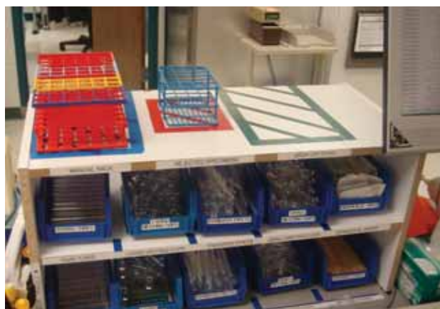
A typical benchtop, now with visual controls, 5S organization, and a two-bin kanban system.
