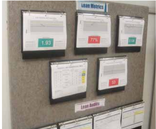
New visual metrics display is updated daily, showing key lab metrics and trends, color coded to show “red, yellow, green” status. Daily supervisor audits of standard work and lean practices are also posted here.
